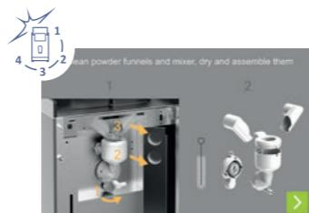
Remove the parts as shown on the display, clean them according to the hygiene concept and reassemble them. Follow the detailed instructions in the "Removal of the instant mixing unit" on the back page.
