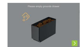
Remove, empty, clean and reinsert the grounds container. After that, press the arrow key to go to the next step.
