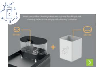
Open the tablet chute and insert a coffee cleaning tablet. Then place a milk cleaning tablet in the empty cleaning container.
