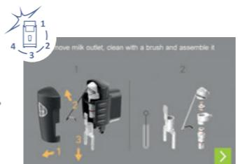
Remove the parts as shown on the display, clean them according to the hygiene concept and reassemble them. Follow the detailed instructions "Removal of the milk outlet / coffee outlet" on the back page.
